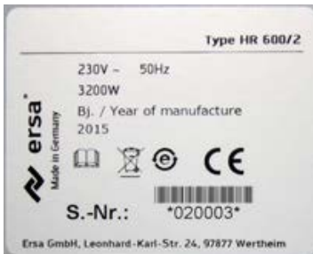
Fig. 61: Example of the nameplate of a machine. The details are not identical to those specified on the nameplate of your machine!
