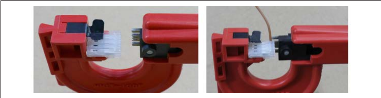
Fig. 20: Example figure. Left: Insertion of the plug-in connector into the crimping tool. Right: Run the cable into the connector pin from above and press the cable in.
