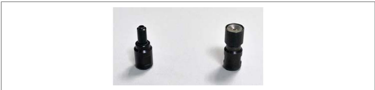
Fig. 61: Example: Heating head nozzle 5 mm left, heating head nozzle 10 mm right
