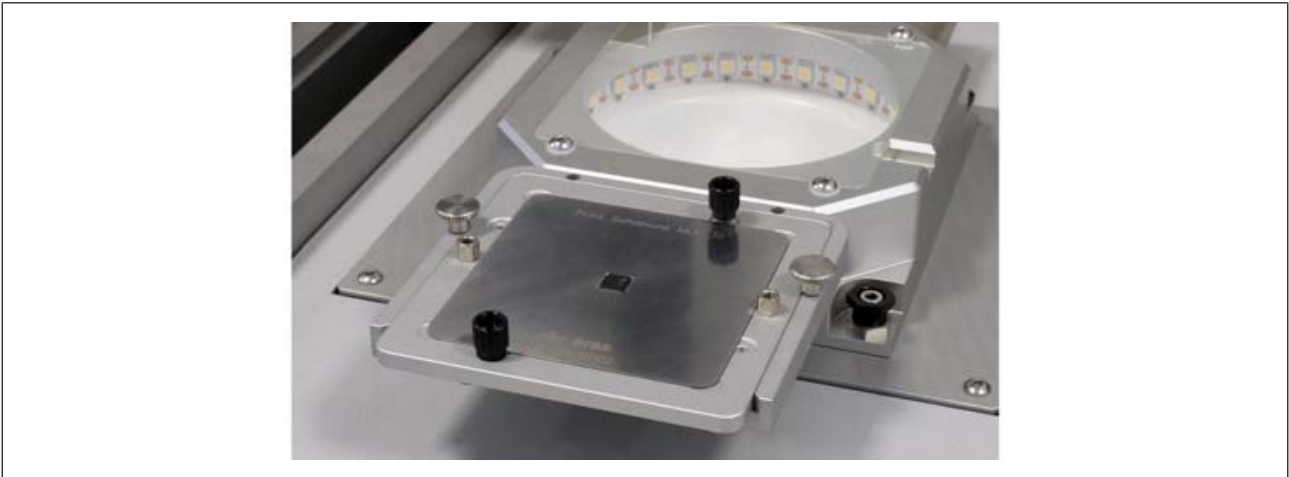
Fig. 46: The solder paste-coated component is inserted into the print stencil and slid into the framed stencil
