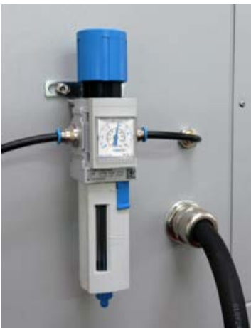
Fig. 21: The maintenance unit
