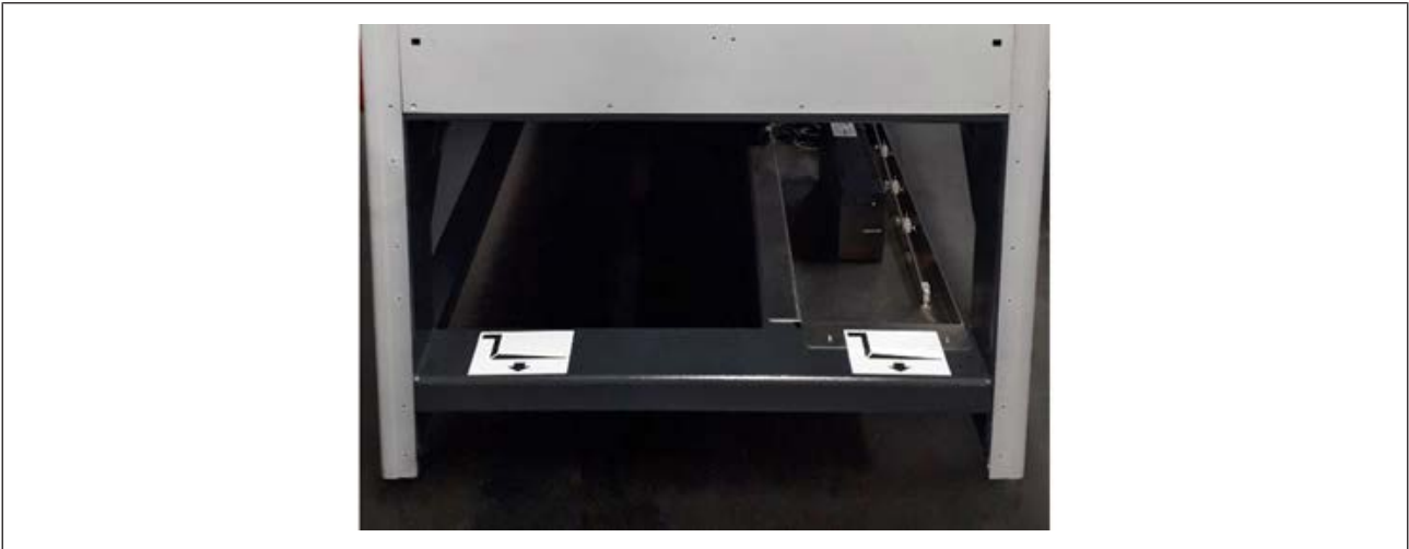
Fig. 6: Lifting points for the forklift
