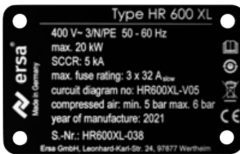
Fig. 51: Example of the nameplate of a machine. The details are not identical to those specified on the nameplate of your machine!
