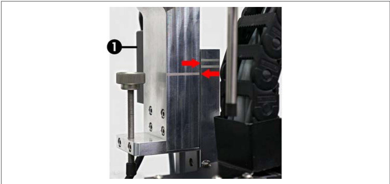
Fig. 25: Arrows: Contour lines for engaging mechanism. (1): Black housing of the engaging hook.
