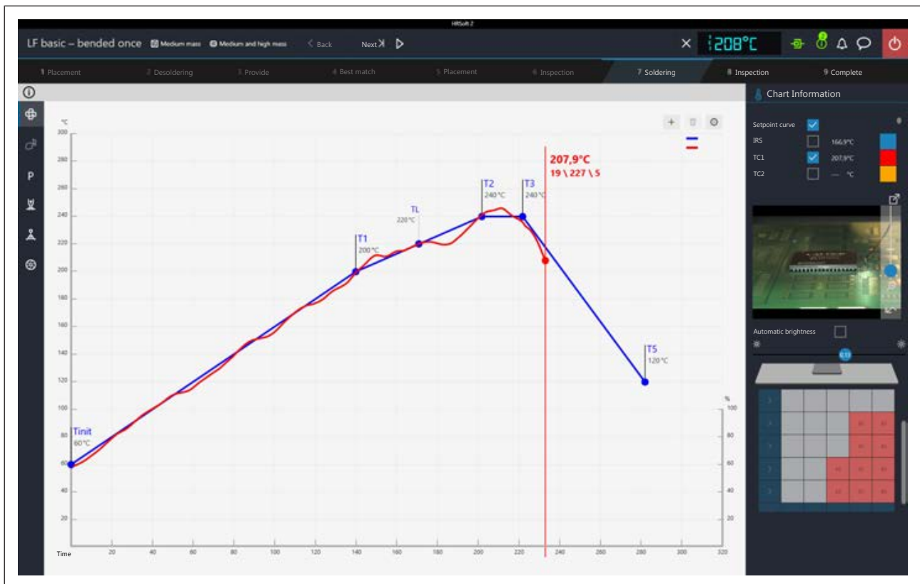
Fig. 50: The chart during cooling after soldering
