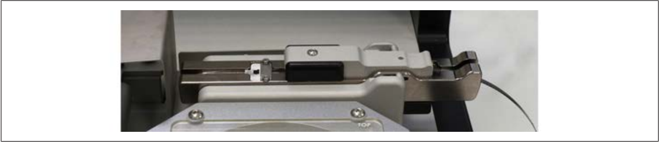
Fig. 40: Tape feeder with the exchangeable assembly for a specific component size, on the basic module
