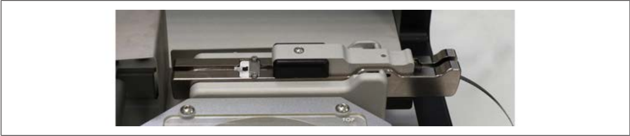
Fig. 41: Tape feeder with exchangeable assembly for a specific component size
