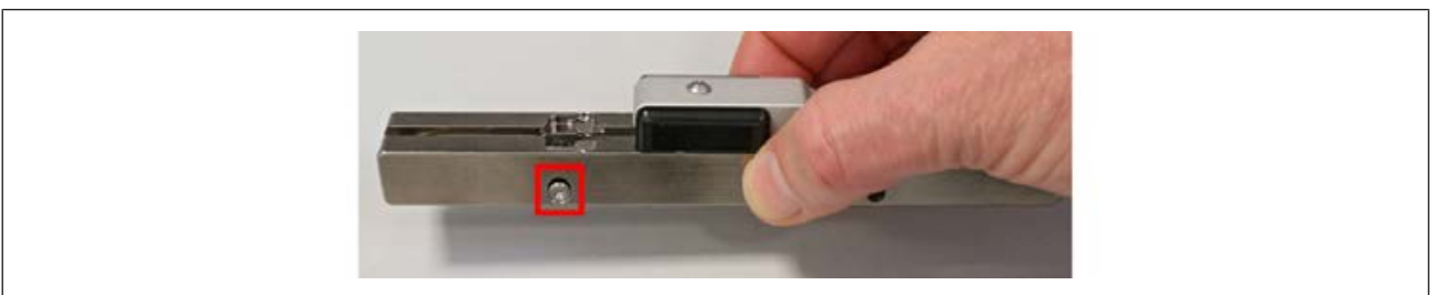
Fig. 47: The lower positioning needle has moved down
