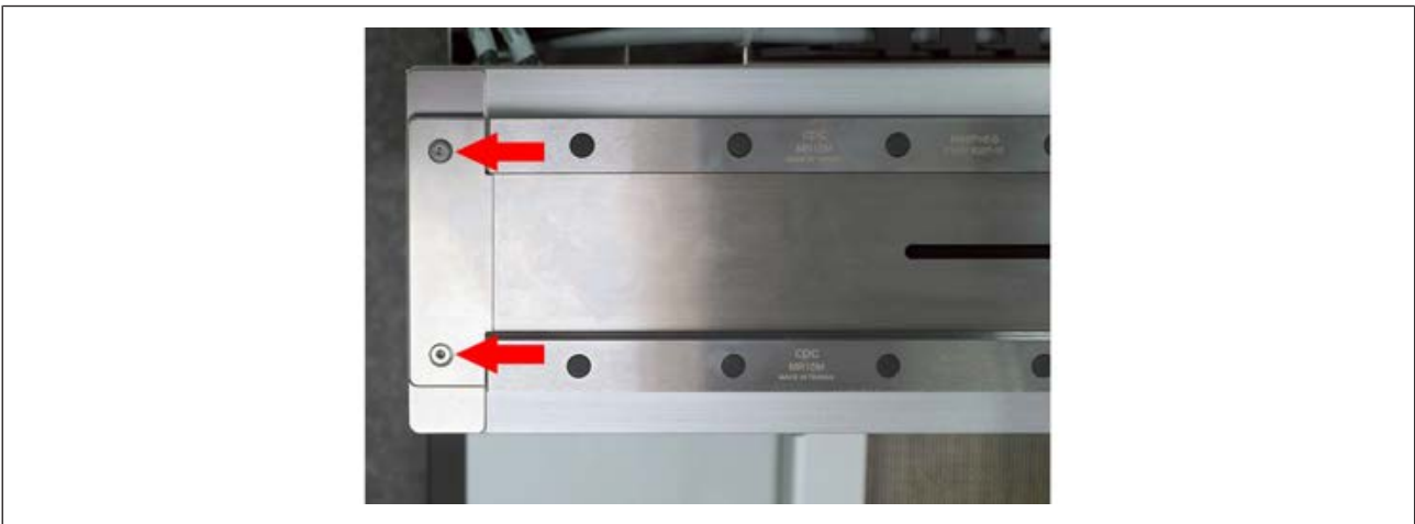
Fig. 36: Removing side end pieces
