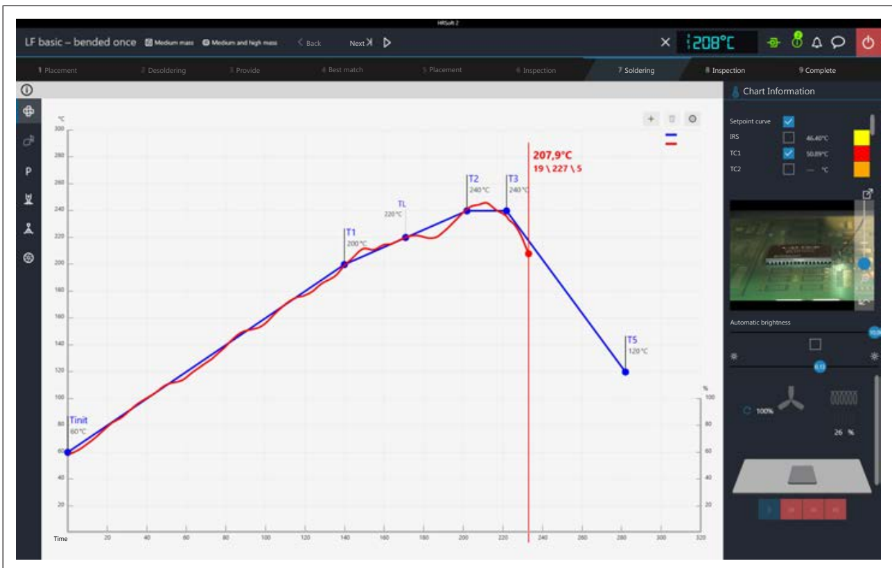
Fig. 33: The chart during cooling after soldering
