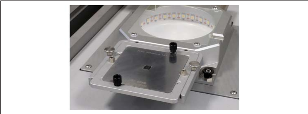
Fig. 29: The solder paste-coated component is inserted into the print stencil and slid into the framed stencil
