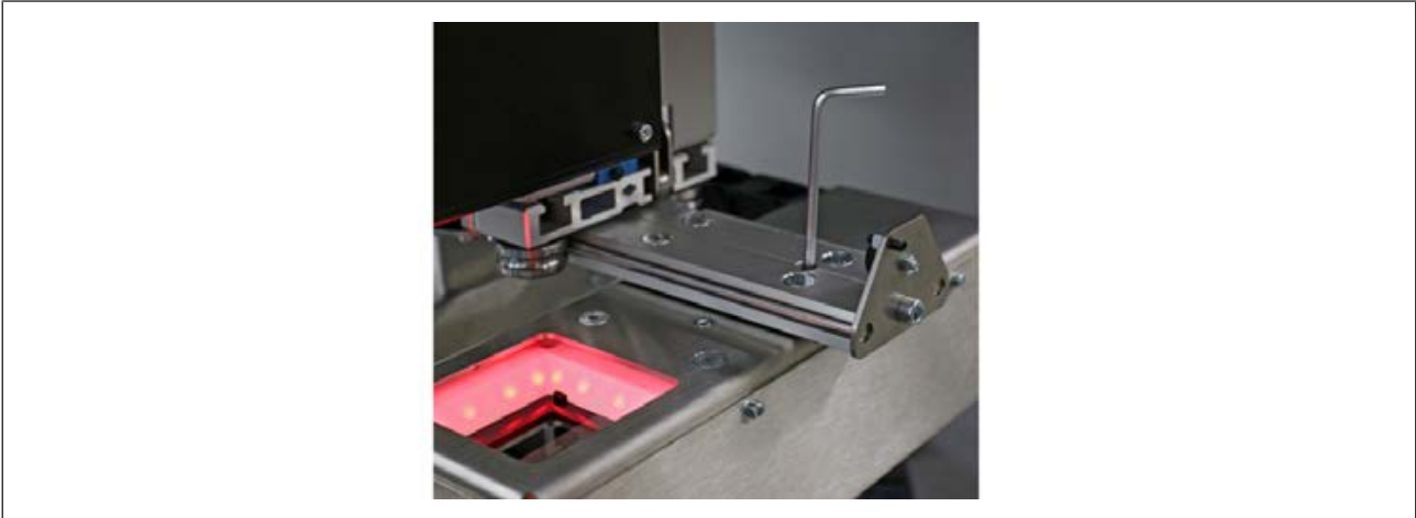
Fig. 14: To correct in Y direction, use a 3 mm Allen wrench. To control the outcome, slide the Visionbox below the camera.
