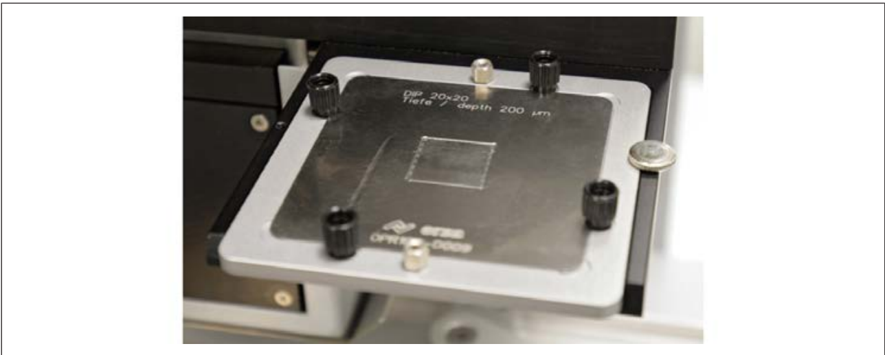
Fig. 38: Dip template covered in flux material on the component tray
