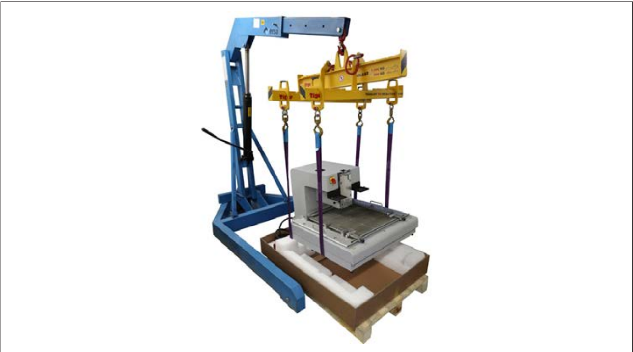
Fig. 4: Lifting the Rework system with a crane
