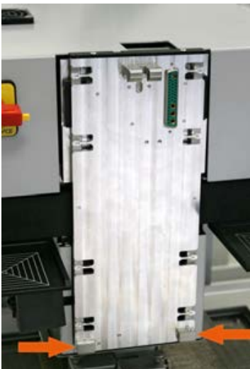
Fig. 48: Heating head suspension bracket, the arrows indicate the supports
