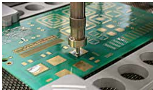
Suction nozzle in operating position
