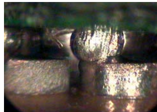
BGA - piggy back: bad alignment
