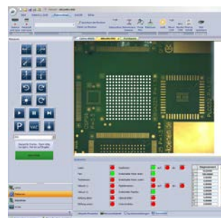
Superimposing of component and target position
