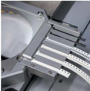
Provision of 01005 components with a tape feeder
