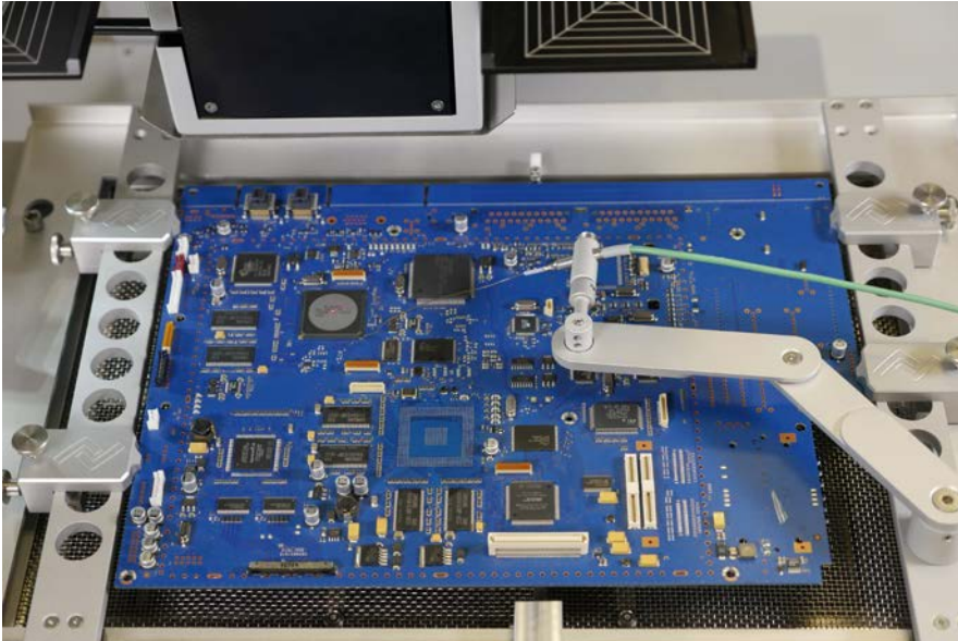
Processing an assembly in the HR 550
