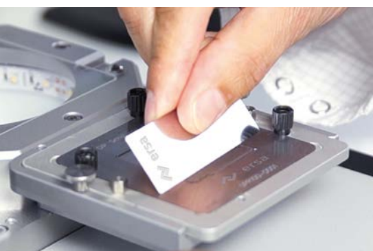
Flux deposition in the dip stencil
