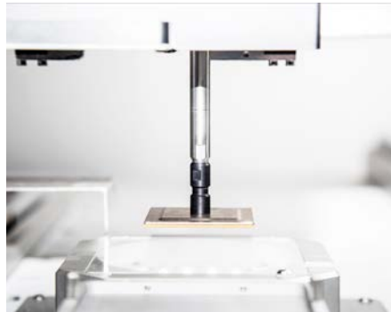
Metallic BGA above the light dome for detection of component connections
