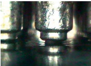
CCGA: insufficient solder
