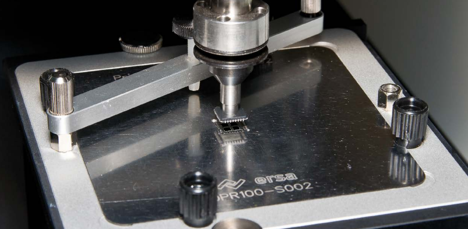
Removal of the component from the print stencil
