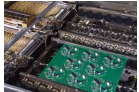
The vacuum module's roller conveyor is free of lubricants.
