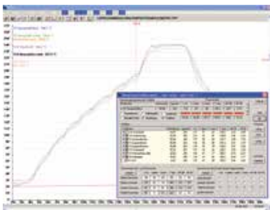
Automatic process evaluation with 6 parameters – Display of gradients with up to 17 profiles
