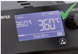
340 – 360 °C for lead-free solder
