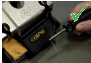
Add new solder after cleaning
