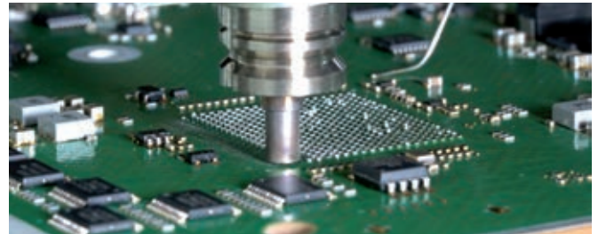
After the component has been automatically lifted off the PCB, remaining solder is removed completely.
