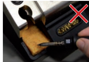
DAMP – NOT WET!
