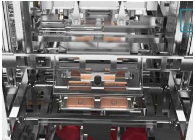
Pick-up of the product carrier by the lift system
