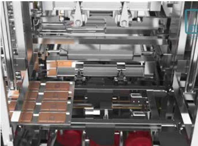
Transport of product carrier to process chamber
