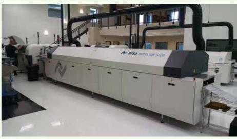
SisTech also places its faith in "best-of-class" results in SMD as well - with a further HOT-FLOW 3/20 reflow system.
