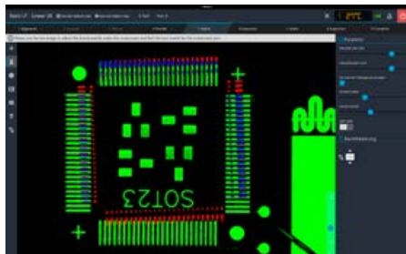
Erska HRSoft 2 – QFP orientation with digital split optic.
