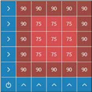
Matrix underheater of the HR 600 XL with warmer edge area
