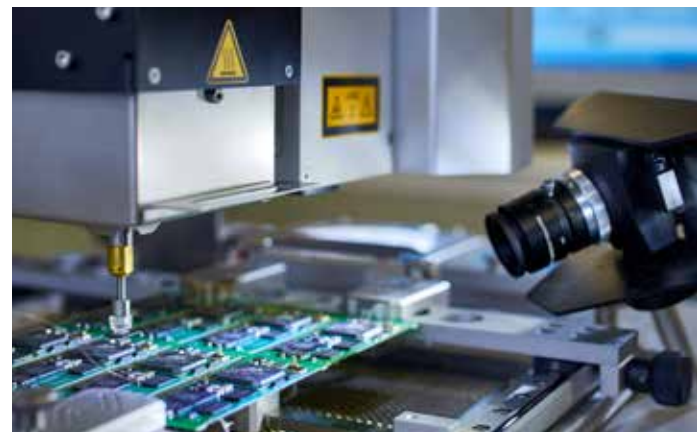
An Erska HR 600 rework system is also used, especially for prototype construction, to maintain the added value of the increasingly complex electronic assemblies
