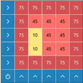
Matrix underheater of the HR 600 XL with "cold spot"
