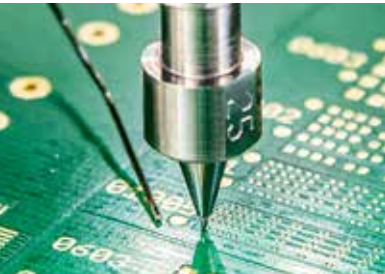
Placement of a 01005 chip with the Erska Hybrid Rework System HR 600/3P
