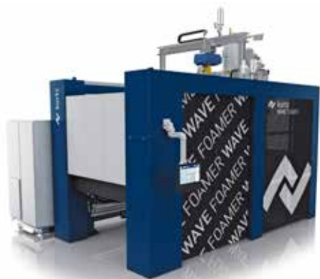
Chemical-free recycling and energy savings of up to 90 %: Kurtz WAVE FOAMER with radiofrequency technology
