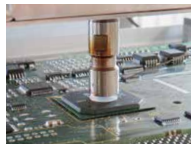
Desolder BGA from controller board
