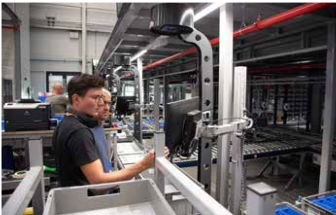
Picking workstations connected via conveyor technology
