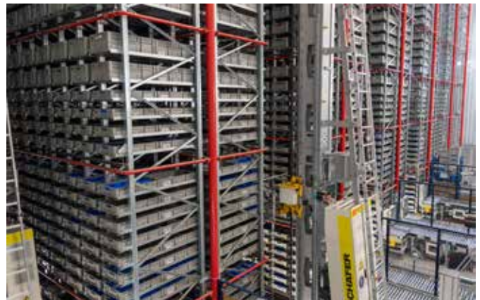
Automated small parts warehouse with control panels
