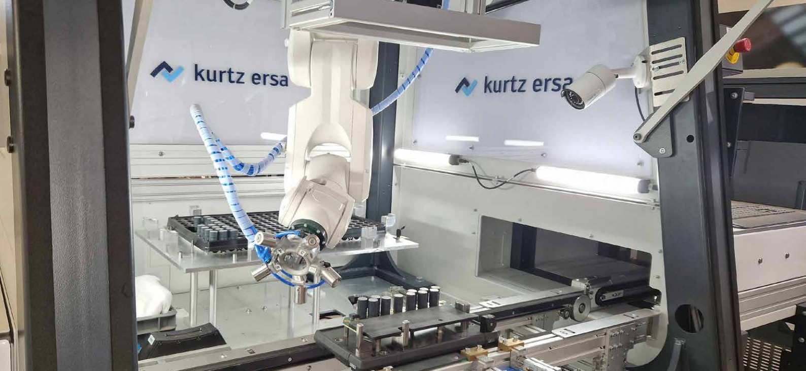
View into the robot cell of the Kurtz Ersä ROBOPLACE during a placement process
