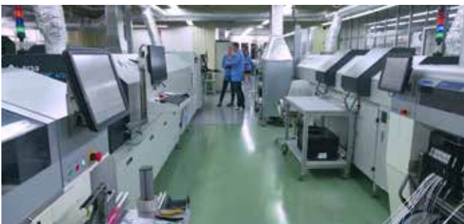
View into the INOTECH electronics production with Ersa reflow soldering systems of the type HOTFLOW 4/14, which is installed three times at the Kaplice location
