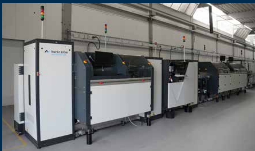
Complete system consisting of brushing station, X-ray station and soldering system
