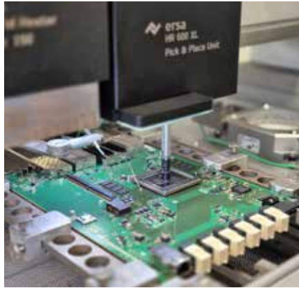
Automatic BGA placement
