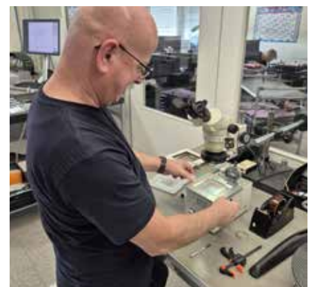
Harald Gillig, Lawo process technician, performing BGA reballing
